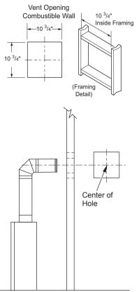
Figure 11 - Vent Opening Requirements
